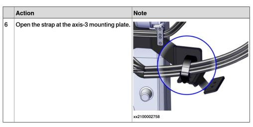
Removing the protection hose (protection type Foundry Plus)
